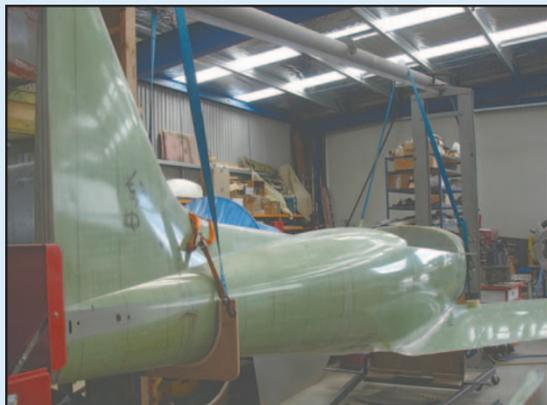
A view of the non-flying fuselage made of fibreglass not carbon to test the infusion process and placement of systems within the airframe.
