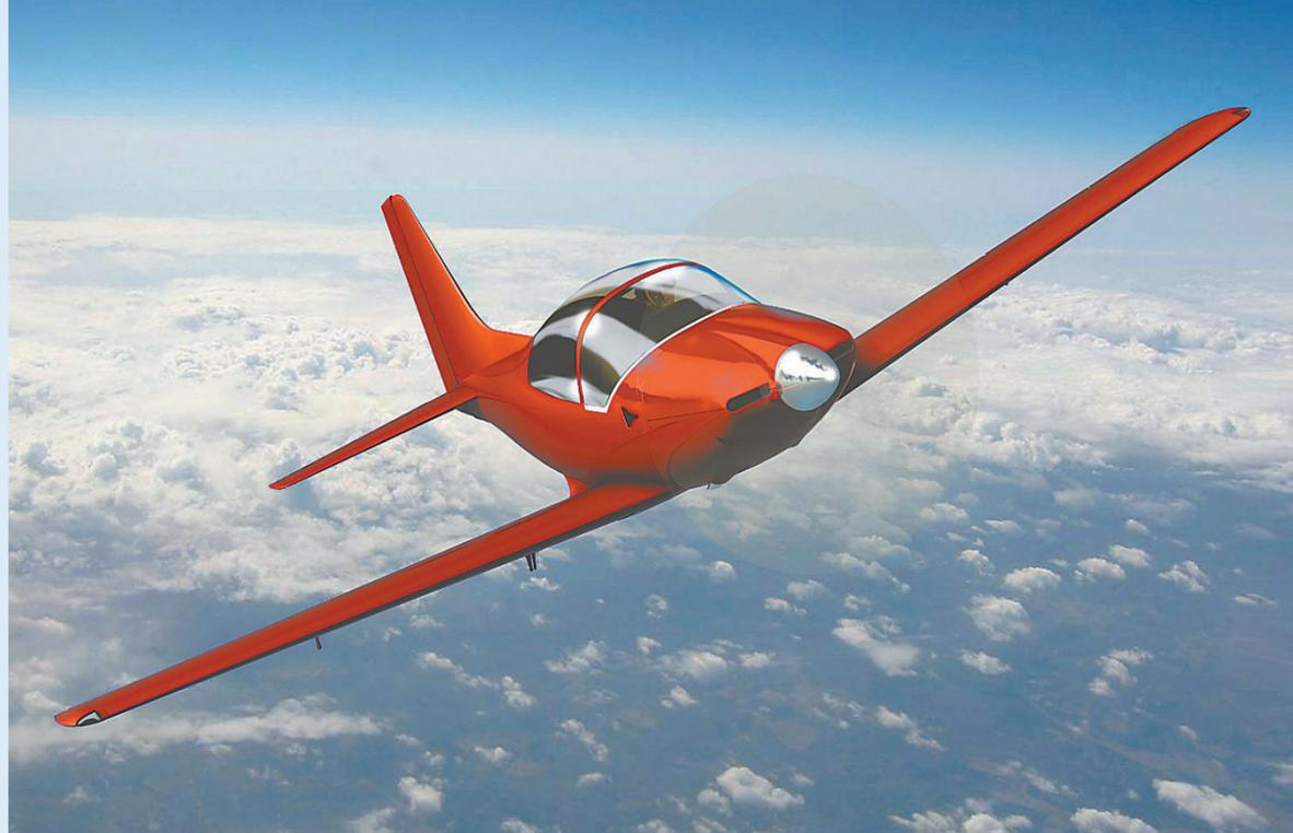
Above: A blend of function following form. Modern composite manufacturing techniques as used in Americas Cup boats results in an airframe containing fewer than 30 major components.
