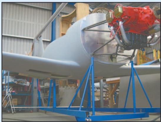
The non-flying fiberglass showing engine mount installation. The initial aircraft will fly with either a Superior XP IO-360 or a Lycoming XIO-360M1A. The engine will drive an MT 3 blade scimitar propeller with constant speed unit.
